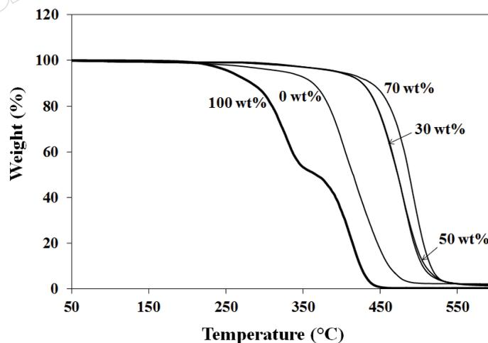
Figure 8 TGA thermograms of the AESO, PMMA and AESO-co-PMMA copolymers.
