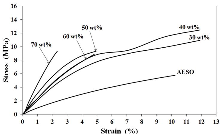
**Figure 3** Stress-strain curves of the AESO, PMMA and AESO-co-PMMA copolymers containing different MMA contents.
