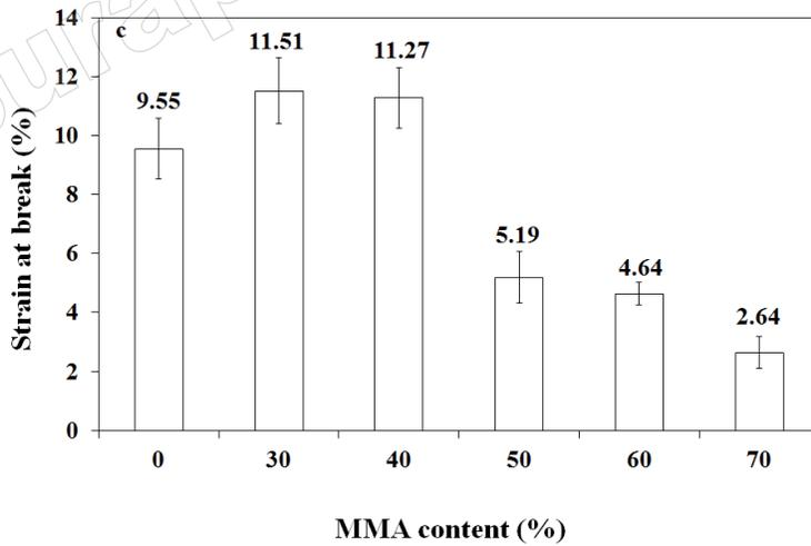
**Figure 4** Effect of the MMA content on the tensile properties of the AESO-co-PMMA copolymers: (a) Young's modulus, (b) tensile strength and (c) strain at break.
