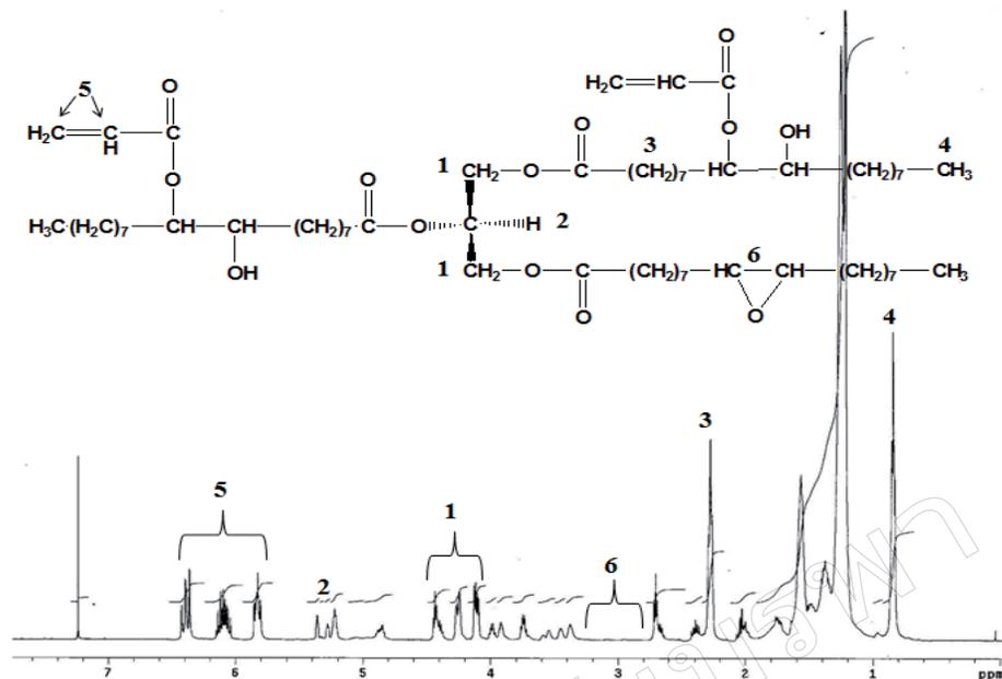
**Figure 1** The  $^1\text{H}$ -NMR spectrum of the AESO showing the acrylate group at position 5.
