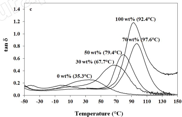
Figure 6 Effect of the MMA content on the dynamic mechanical thermal properties of the AESO-co-PMMA copolymers: (a) storage modulus, (b) loss modulus and (c)  $\tan \delta$ .
