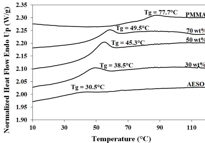
Figure 7 DSC thermograms of the AESO, PMMA and AESO-co-PMMA copolymers.
