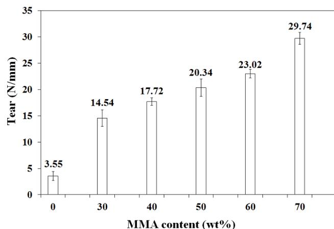
**Figure 5** Effect of the MMA content on the tear resistance of the AESO-co-PMMA copolymers.
