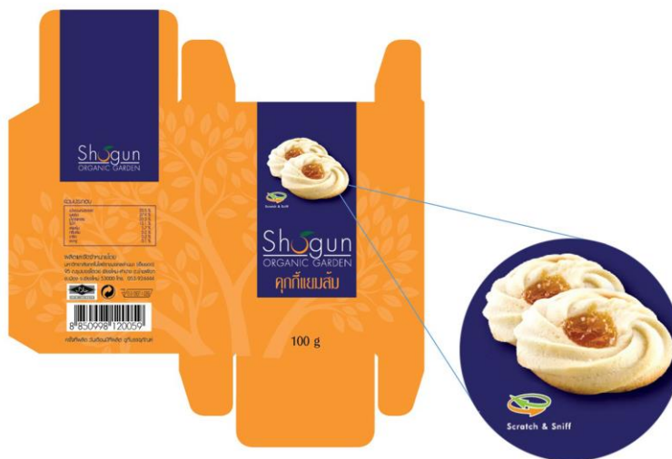
Figure 1 The region on cookie box was designed for spot coating with orange essential oil microcapsule
