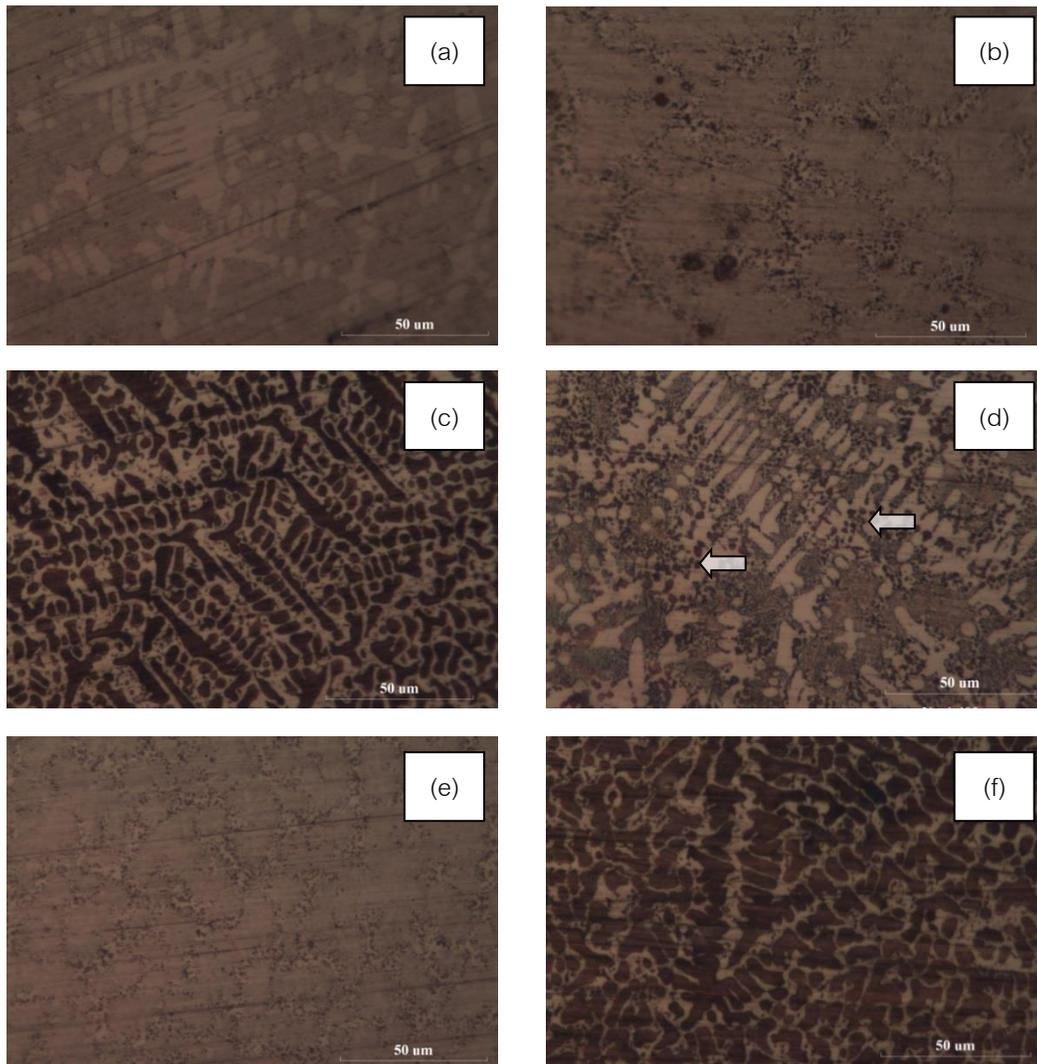
**Figure 1** Light micrographs of (a) A1 sample, (b) A2 sample, (c) A3 sample, (d) A4 sample, (e) A5 sample and (f) A6 sample and white arrows are intermetallic phases. (Etchant: chromic acid)
