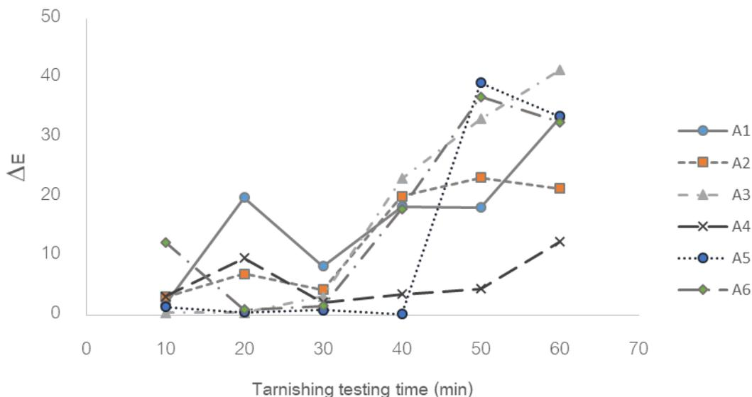
Figure 4 Color difference of samples after tarnish test
