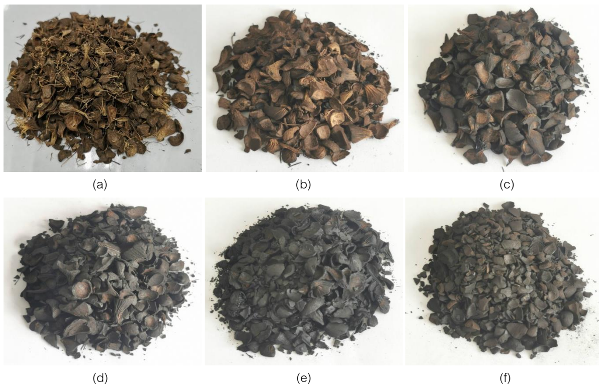
Figure 2 Physical characteristics of palm kernel shell (a) and torrefied palm kernel shell at 300 °C for durations of (b) 100, (c) 200, (d) 300, (e) 400, and (f) 500 seconds.
